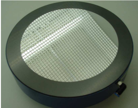
Figure 3.21: Photo of the aluminium coated, \varnothing 150\text{mm} Pyrex mirror facesheet placed on the \varnothing 200\text{mm} air bearing. The filter of the air flow cabin is visible in reflection.
