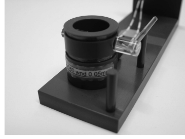
Figure A.3: The rotation table within the Ø15mm coils with its end stops is visible.
