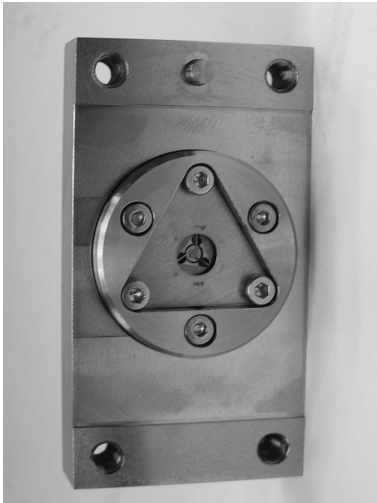
Figure B.6: The actuator placed in the container
