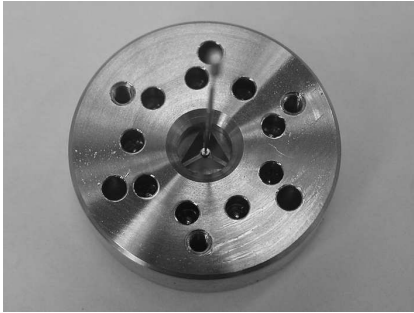
Figure B.4: Photo of the container with membrane suspension.
