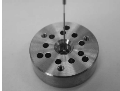
Figure B.5: The strut that connects the membrane suspension to the force sensor is clearly visible.
