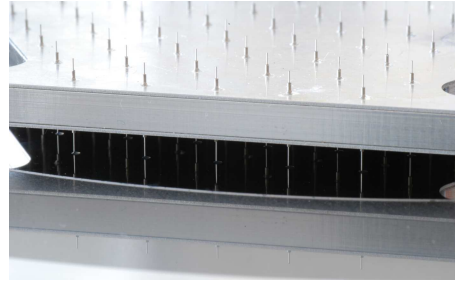
Figure 3.28: Photo of a few struts guided by the needle tubes while placed in the glue droplets.
